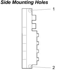
The mounting materials required are two screws with a diameter of 4 mm (M4, 0.157 in.) and a maximum head diameter of 7mm (0.276 in.) and two retaining washers. The length of the screws depends on the mounting method used (at least 30mm [1.181 in.] for front mounting, at least 40mm [1.575 in.] for side mounting). The tightening torque is 0.8Nm.
