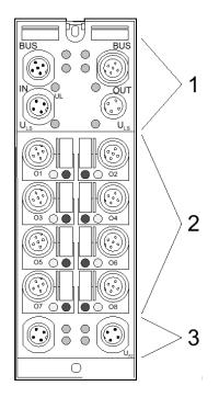
Diagnostic LEDs (green/red) indicate whether an error is present or not. In the event of an error, they indicate the error type and location. The VersaMax IP module is functioning correctly if all of the green LEDs are on.
