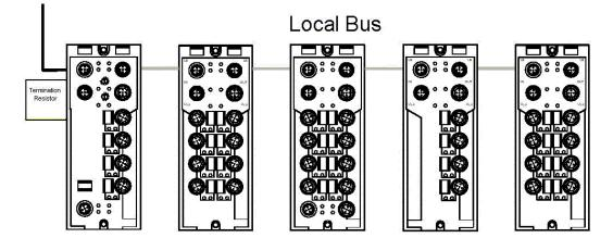
The maximum total length of a local bus is 20 m. The transmission speed can be switched from 500 Kbaud to 2 MBaud.
