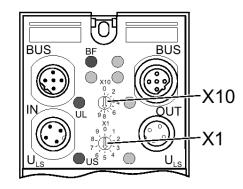
Adjust the rotary switches using a suitable screwdriver (blade width 3.5mm [0.138 in.]). Use of an unsuitable tool may damage the rotary encoding switches.
