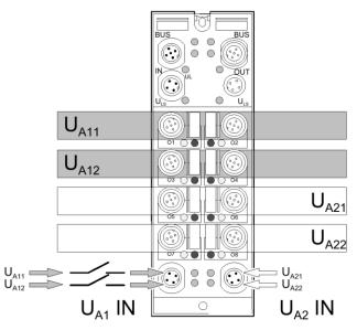
If you switch off the voltage  $U_{A11}/U_{A12}$  in the example, outputs O1 to O4 are switched off. Outputs O5 to O8 can still be operated independently.
