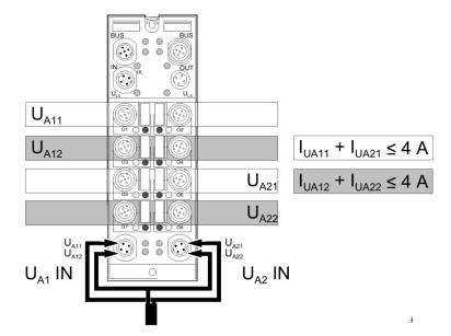
Example 2: Optional Supply via a Y Cable with Reduced Current, VersaMax IP Standalone Only
