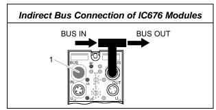
Indirect connection allows devices to be removed or added while the bus is running without physical interruption. To do this, the master and the control program must support the removal and addition of devices. All transmission rates are supported.
