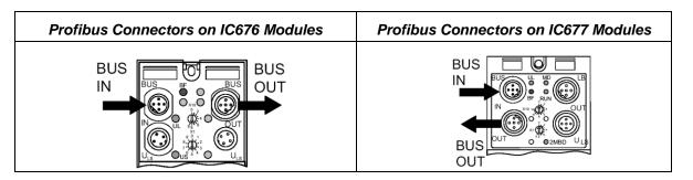
VersaMax IP Standalone (IC676) modules can also be connected indirectly, using a T-connector attached to the module's BUS OUT connector. This requires a Tconnector (IC676ACC005), and one protective cap (IC676ACC002). Transmission speeds above 1.5 Mbaud require T-connectors with integrated series inductance. To ensure IP65/IP67 protection, cover the unused BUS IN connection on the module with the protective cap (1, below right).
