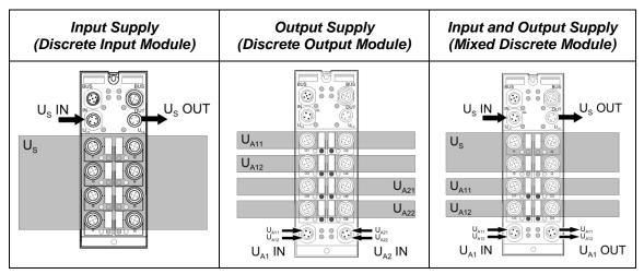
The diagrams below show which VersaMax IP Modular (IC677) module inputs and outputs are supplied by each supply voltage. See the module datasheets in appendix A for details of connecting sensors and actuators.
