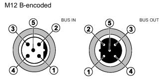
The thread is used for shielding.
