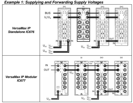
The connection for the outgoing supply voltage is not monitored for overload. If the 4A permissible current-carrying capacity is exceeded, it may lead to connector damage.
