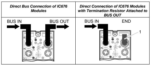
The termination resistor can be attached to BUS OUT on the module (1, below left). A termination resistor can also be attached to the open connection of a T-connector (1, below right). When using a T-connector, cover the unused BUS IN connector on the module with a protective cap (2, below right) to ensure IP65/IP67 protection.
