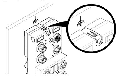
If the module is mounted on an ungrounded mounting surface (as shown below) or sidemounted, the module must be grounded using lugs (2.8 mm [0.110 in.]) via the external grounding connection (connection latch).
