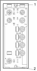
For direct mounting on the front on a grounded mounting surface, the devices are grounded using the upper mounting screw.
